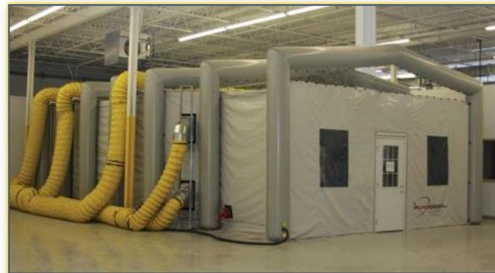
Figure 1. Inflamm's patented Mobile Environmental Exposure Unit (MEU)™ with environmental controls of temp, Rh and allergen
